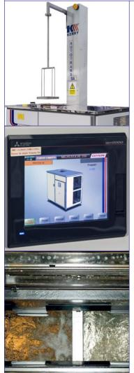
The Kerry Microsolve Mono-Solvent system manufactured by Guyson has three process stages comprising of ultrasonic cleaning, followed by vapour rinsing and freeboard drying. The Microsolve has unique proven solvent retention features that provide economic benefits as well as effective use of HFE (hydrofluoroether) or HFC (hydrofluorocarbon) solvents.
