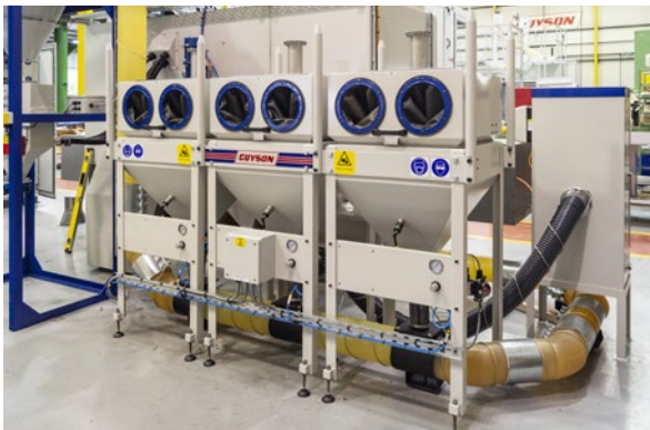
Above: Mesh belt In-Line blast system with oscillating guns for full belt width blast coverage and incorporating a three blast media grade auto-top-up system
