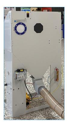
Left: Rear of Formula 1400 CCR cabinet showing ionised air power box, busbar for earthing, quick release breather pad filter
