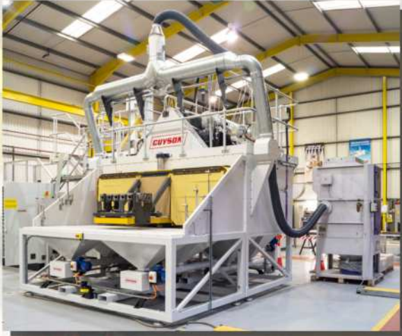
Dual Robotic Blast Carousel Table ID Special Purpose Lance Blasting
