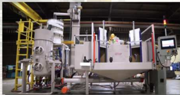
Multiblast RXS1400 AMS 2432 Shot Peening Turbine Blade Roots & Gears
