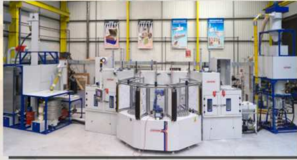
Multiblast RXS900 Dual Shot & Glass Bead Peening
