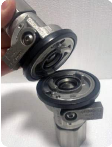
01 Align the lugs with the grooves on the mating coupling.
