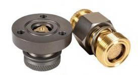
Danfoss Hansen LF series is a specific coupling made for industrial applications using SF6 gas. Its design allows a perfect sealing over several decades and an extremely limited permeation of media into the atmosphere during connection and disconnection, in order to limit global warming. The coupling has a dual O-ring design and dust caps ensuring tight sealing while it is disconnected
